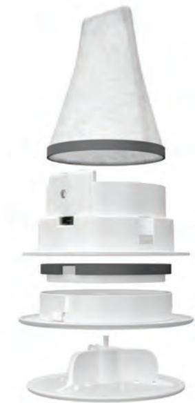
The filter can be quickly replaced by simply removing the damper assembly and changing the filter. The damper assembly is then put back into its place without any adjustment of the commissioned set point, thus ensuring the system remains commissioned.
