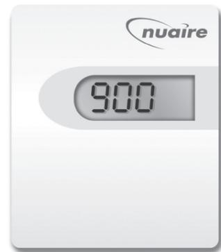
As the room CO2 and temperature rises, the fan speed will progressively increase in steps until the upper threshold values are reached. When both CO2 and temperature readings are in operation, whichever reading that results in higher fan speed will be used by the fan unit.
