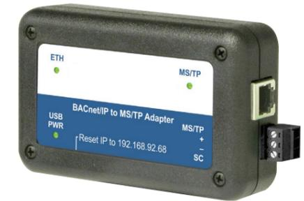
The BACnet router has a USB 2.0, Type B receptacle which is only used to obtain power from a computer or USB adapter. A mains adapter and cable is supplied. The router connects to the FC bus via screwed terminals.
