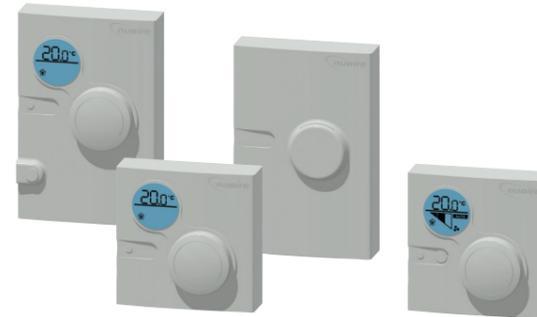
Room modules are automatically detected and require no set-up. The majority of RM modules monitor room temperature; however, options are available to also monitor zone humidity, carbon dioxide (CO2), local temperature setpoint adjustments, PIR, and other variables. This data is transmitted to a controller on the Sensor Actuator (SA) Bus.
