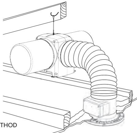
STANDARD METHOD OF FIXING
