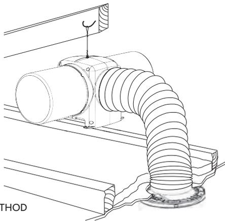
STANDARD METHOD OF FIXING
