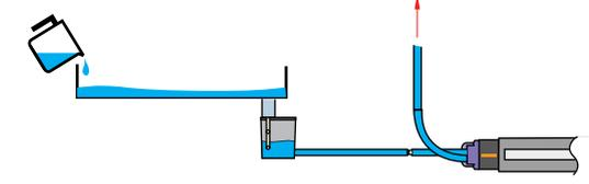
To ensure that the alarm connection is working, restrict the outlet of the reservoir/DrainStik™ hose and fill with water up to the high level sensor. The pump will turn on initially, then after a short delay the alarm relay will switch, detected using a multimeter or observing the shut down of the AC unit. Allow the water to exit the reservoir; the water should then be pumped away, and AC operation will restart.
