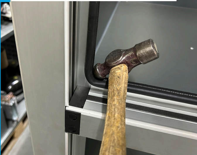
3 Hammer the Sealing Strip into Each of the Corners.
