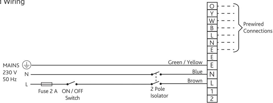
5 Single Speed Wiring with Mains Activated Back-draught Damper
