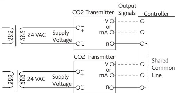
If several sensors share one transformer, the phase (~) must always be the same at each sensor to maintain polarity and avoid a short circuit via a shared common line at the controller, as shown in Figure 3.
