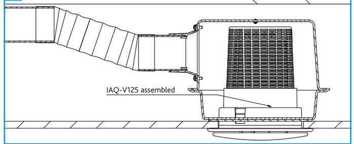
3.3 Fitting the Airflow Screen
