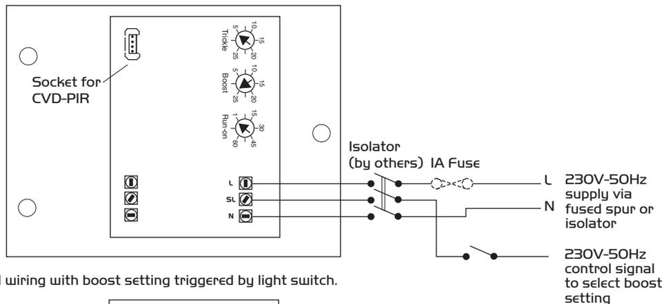
Figure 8. Typical wiring with boost setting triggered by light switch.
