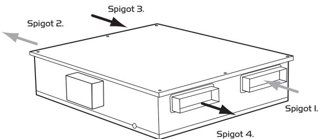
**Note:** The unit must be installed in an upright position as shown for the condensate drain and for compliance with safety regulations relating to IP protection for water drip ingress.
