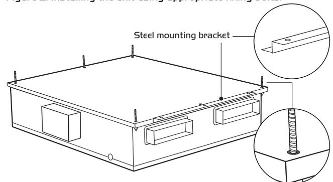
Figure 3. Typical side view example of a unit mounted in a ceiling void using 204 x 60mm rectangular ducting and air valves.
