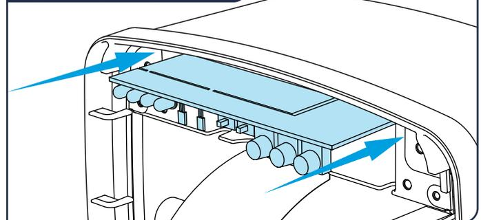
**5.2.3 SEMI-RECESSED FAN INSTALLATION PROCEDURE**
