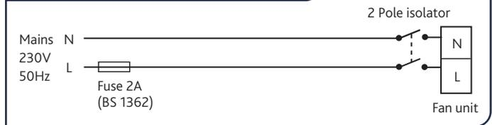
**4.3 WIRING DIAGRAMS - 230V TWO ROOMS VIA SIDE SPIGOT**
