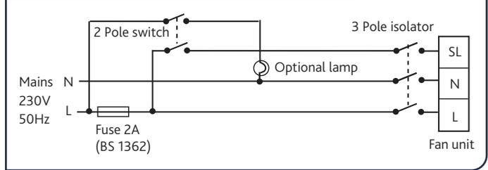
**Fig 15: Wiring - 230V via Pull Cord**
