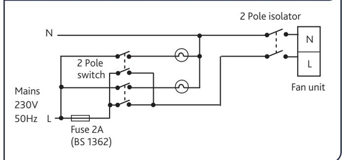
**Fig 17: Wiring - 230V Two Rooms via Pull Cords**
