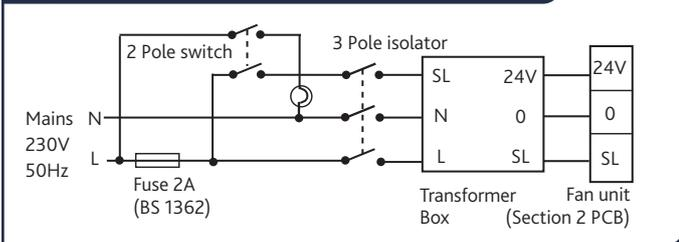
**Fig 13: Wiring - 24V SELV via Pull Cord**
