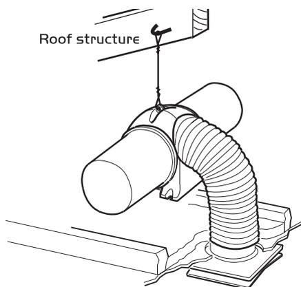
The method of locating the wire to the roof timber is the responsibility of the installer.
