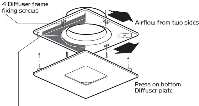
2 Foam strips (supplied) fit on any of the diffuser sides to guide airflow away from a smoke detector and/or obstructions as required.
