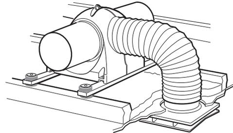
Place anti-vibration mounts (supplied) above and below each batten fixing point and, using the 4 large screws and special washers, fix the unit to the joists.
