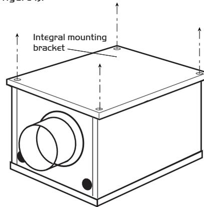
Please note that a clear space of at least 470 x 320mm is required to allow the cover to be removed and provide sufficient access for maintenance.
