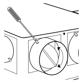
Various damper/inlet spigot positions can be utilised as required to suit the system ductwork and extract grilles as all spigot positions are removable. After the spigots has been located in their correct position, adjust the damper with a screwdriver. (See figure 4).
