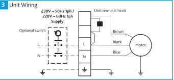
Check the fan voltage and circuit details are compatible with the power supply. Wiring must comply with appropriate regulations including any requirements of the local supply authority.
