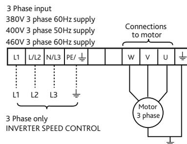
Note: Screened cable must be used. Maximum length should be 30m and must be earthed at both ends and continually earthed through any insulators.
