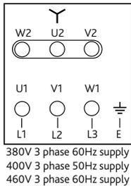
Figure 6. 3 phase units 4kW and above.
