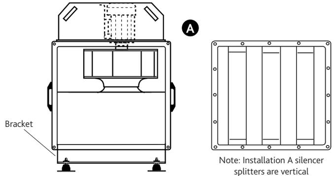
Figure 3. End view of non-recommended horizontally mounted unit installation (bracket by others).
