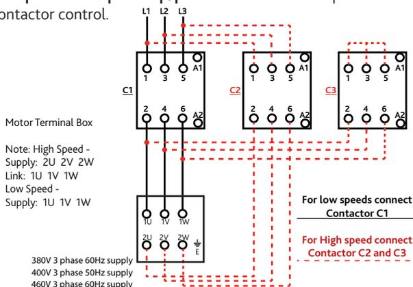
3 phase Dual wound motors require a two contactor control.
