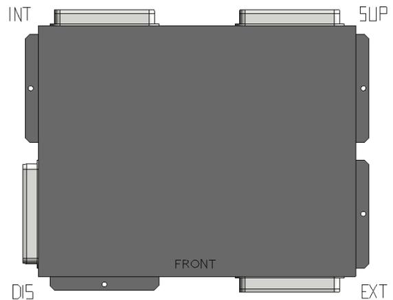
2. 'Hide Bottom Spigots' is there for when the unit is to be close coupled to the main MRXBOXAB-ECO4 unit. In this situation the ECO4's spigots will pass into the first fix box.
